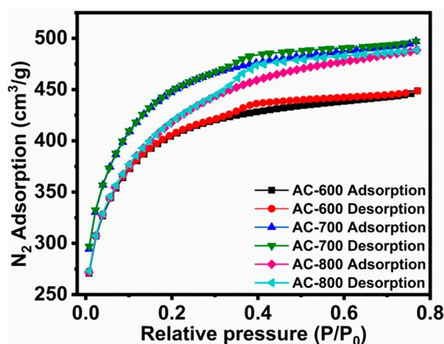
Figure 2. N<sub>2</sub> Adsorption-desorption isotherms of activated carbons.
