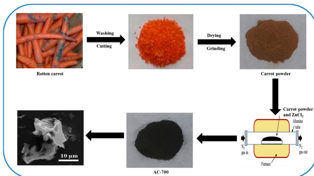
**Scheme 2.** The fabrication processes of activated carbon.
