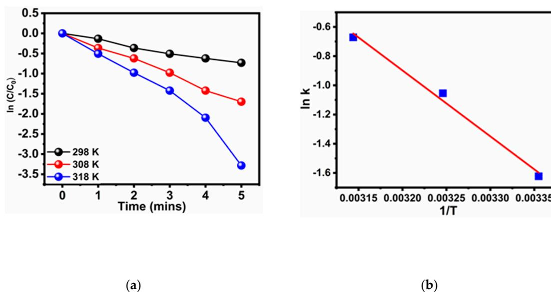
**Figure 5.** (a)  $\ln C/C_0$  versus time curve for the degradation of RhB in the presence of AC-700 at different temperature and (b) Arrhenius plot ( $\ln k$  versus  $1/T$  curve).
