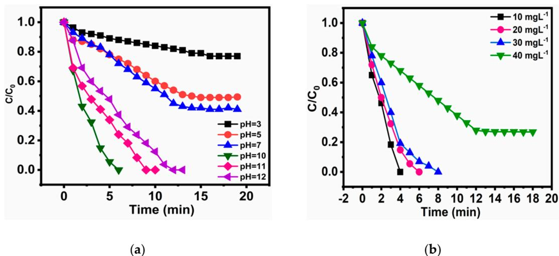
**Figure 4.** (a)  $C/C_0$  versus time curve for the degradation of RhB with different concentration dye in the presence of AC-700 and (b)  $C/C_0$  versus time curve for the degradation of RhB at different pH.
