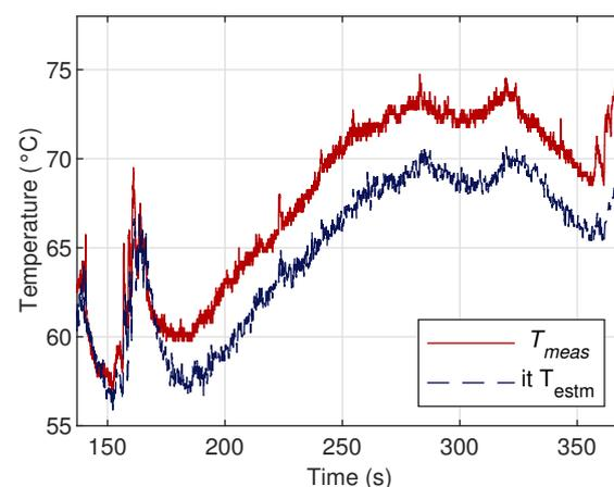
**Figure 17.** Measured temperatures and simulated temperatures of the smartphone while put in a heated environment. Divergence starts around  $t = 190$  s.
