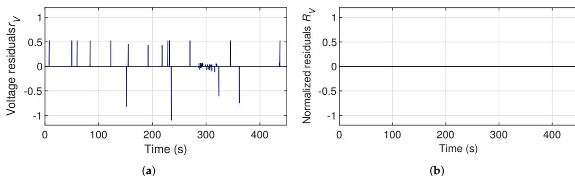
**Figure 12.** Profile of the residuals  $r_v$  and  $R_v$  during normal operation scenario: (a) raw residuals  $r_v$ , (b) normalized residuals  $R_v$ .
