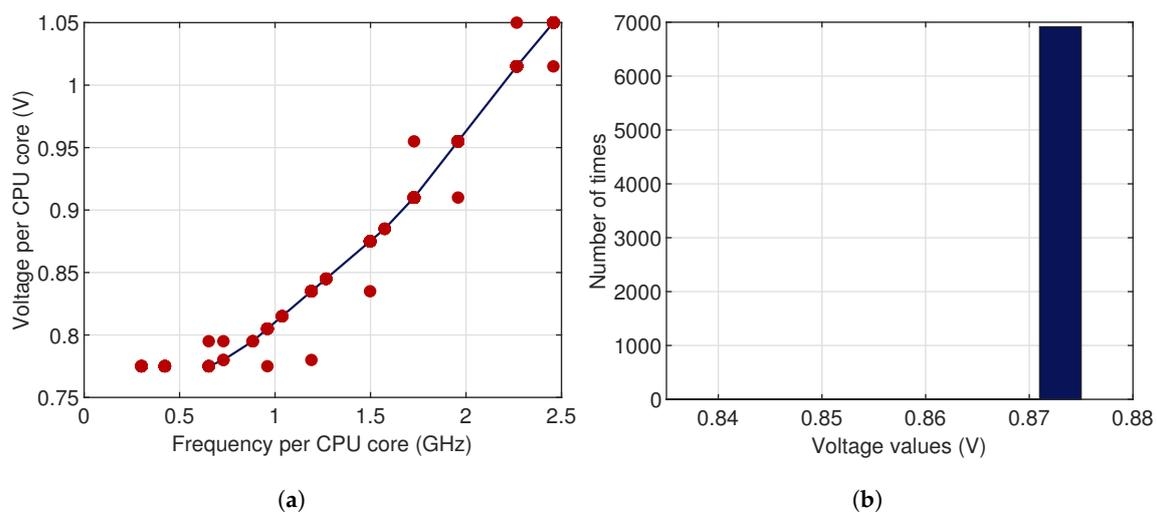
**Figure 6.** Frequency vs. voltage for the Samsung Galaxy S5 Central Processing Unit (CPU). (a) The voltage values drawn against the frequency values (in red), show a quasi-linear trend (in blue). (b) A histogram of voltage values for  $f = 1.49$  GHz.
