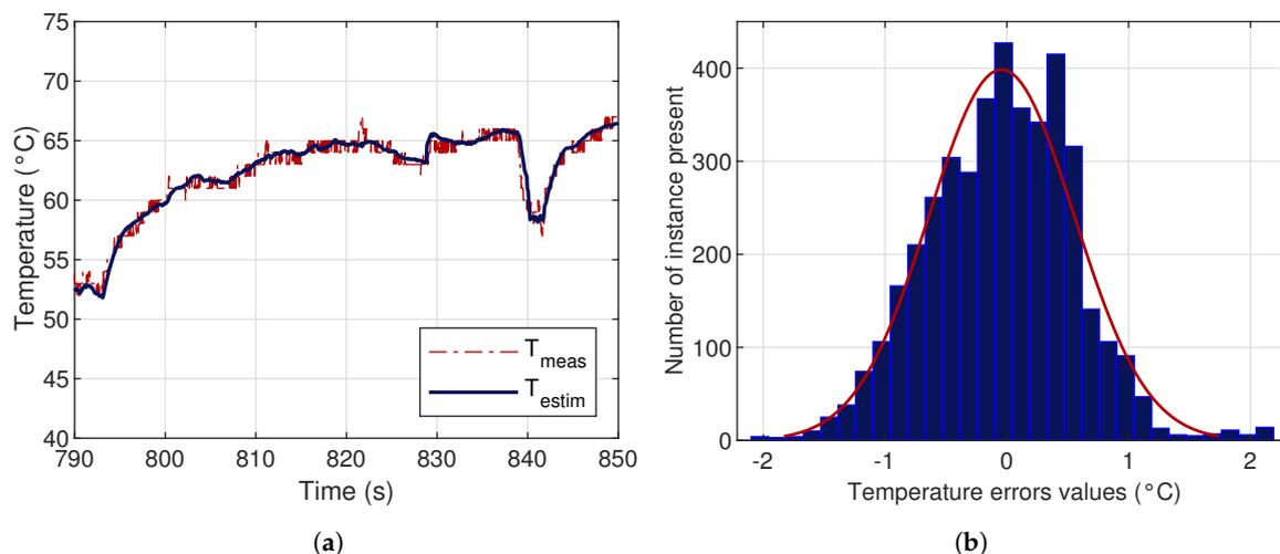
**Figure 10.** The Autoregressive–Moving-Average with Exogenous Inputs (ARMAX) temperature model performance. (a) ARMAX model temperature estimations compared to system readings. (b) Distribution of the ARMAX Temperature estimation errors.
