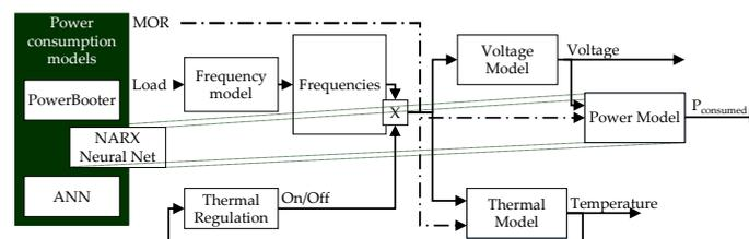
**Figure 2.** The incremental structure of the general model makes very simple to adapt it to changes in the structure and even exchange components at will. ANN: Artificial neural network. NARX: Nonlinear Autoregressive with eXogenous input.
