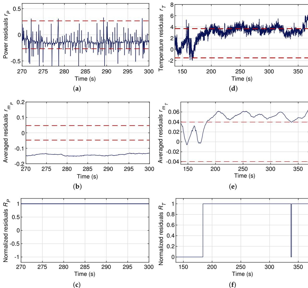
**Figure 18.** Power residuals assessment during faulty scenario of the introduction of an external component, and temperature residuals during the heating experiment. (a) Power raw residuals  $r_p$ . (b) Power averaged residuals  $r_{m_p}$ . (c) Power normalized residuals  $R_p$ . (d) Temperature raw residuals  $r_T$ . (e) Temperature averaged residuals  $r_{m_T}$ . (f) Temperature normalized residuals  $R_T$ .
