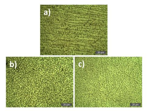
**Figure 6.** Microstructure of sintered Co pellets (700 °C) for sets (**a**) I, (**b**) II, (**c**) III of Co powders as determined through optical microscopy.
