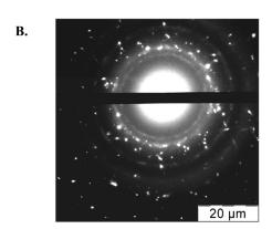
**Figure 1.** (A) X-ray diffraction (Cu K $\alpha$ ), and (B) selected area electron diffraction (SAED) results on synthesized Co nanopowders.
