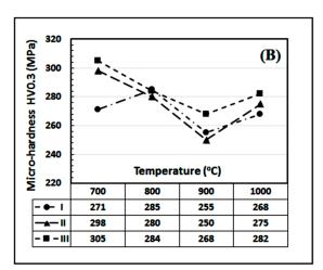
**Figure 8.** Impact of pre-treatments and sintering temperatures on **(A)** bending strength and **(B)** microhardness of sintered pellets.
