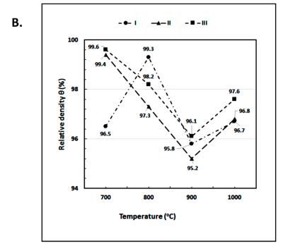
**Figure 7.** Influence of sintering temperature on **(A)** absolute densities and **(B)** relative densities of three sets of Co powders.
