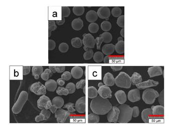
Figure 3. SEM images of Co powders after HEMT operation. (a)  $t = 0 \min$ , (b)  $t = 1 \min$ , (c)  $t = 2 \min$ .
