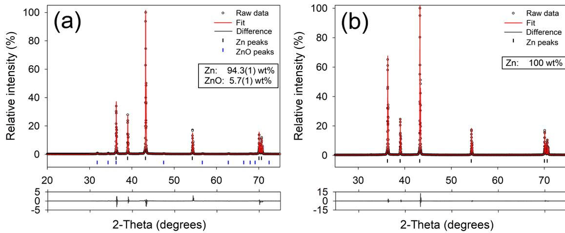
**Figure S3.** Fitted x-ray diffractograms of as-received (a) Zn powder and (b) Zn foil. A strong degree of preferred orientation was observed for the Zn foil sample, and corrected for using a spherical harmonics type correction function
