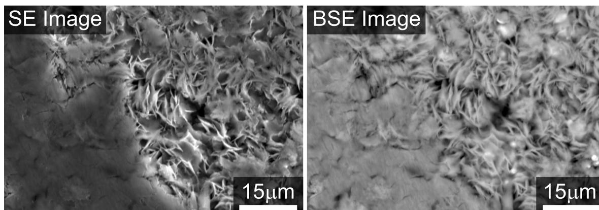
Figure S2. Secondary Electron (SE) and Backscattered Electron (BSE) images of a porous Zn monolith after reaction with acetic acid
