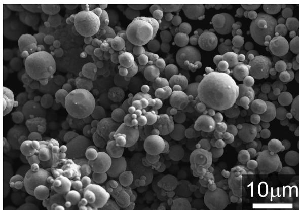
Figure S1. Secondary Electron (SE) image of initial Zn powder
