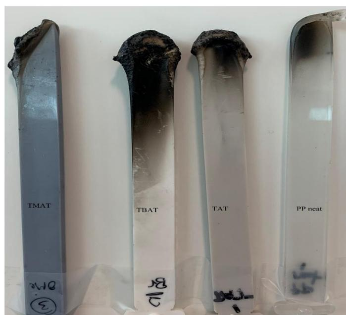
**Figure 4.** PP1, PP2, and PP3 specimens after UL94 tests.
