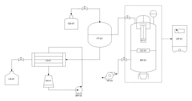
**Figure 1.** Modified vacuum pyrolysis diagram for converting bagasse to syngas. CC-01: biomass chamber; CP-01: control panel; CD-01: condenser; EC-01: electromagnetic induction source; FT-01: flash tank; GS-01: gas storage; LS-01: liquid storage; RP-01: pyrolysis reactor; VP-01: vacuum pump; WD-01: water drum; and WP-01: centrifugal pump.
