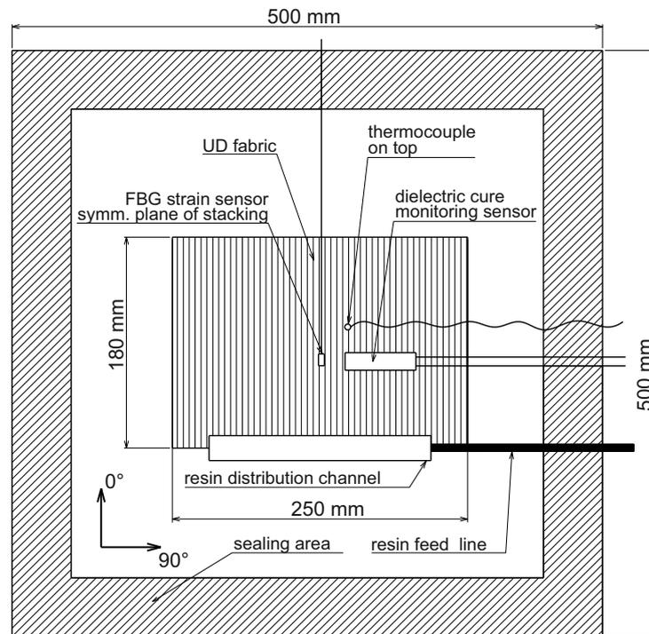
Figure 1. Sketch of the experimental set-up.
