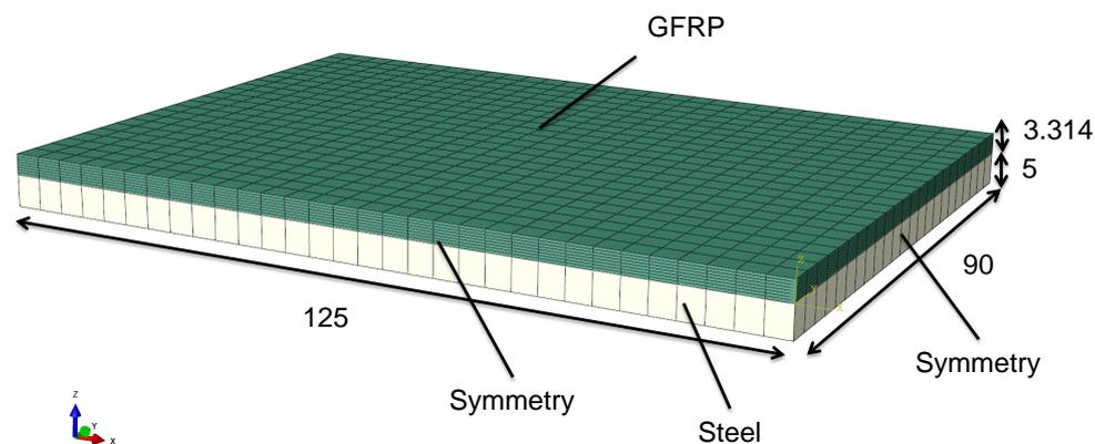
**Figure 10.** FE-Model of laminate.
