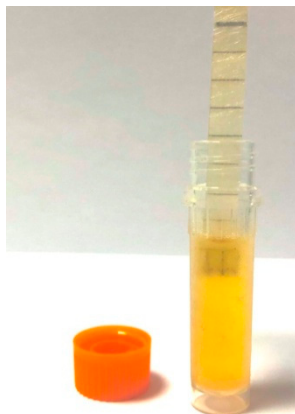
Figure 1. Procedure for filling the membrane carrier with a blood plasma sample.
