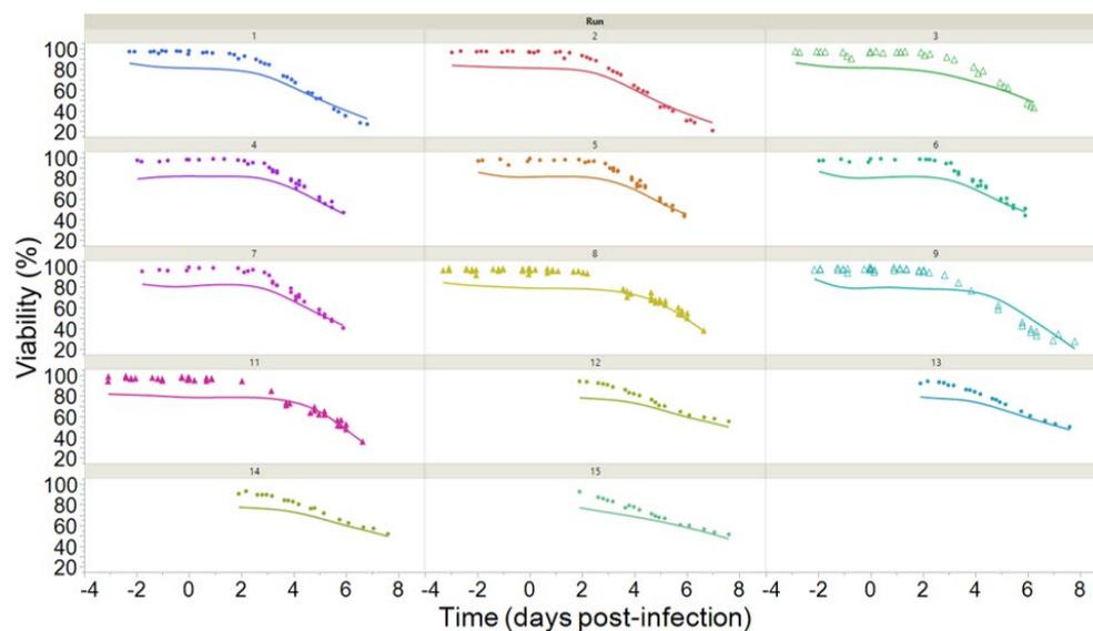
**Figure S1** - Viability reference data and corresponding predictions using only the conductivity data. For each run, a linear fit was obtained between conductivity and viability, considering only the data after viability started to decrease. This simple fit can be applied in the process-to-target.
