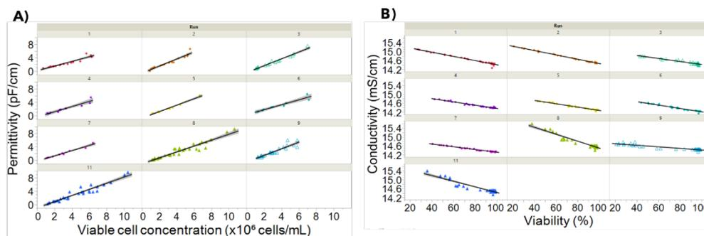
**Figure S3** - Linear correlation between permittivity and viable cell concentration (A) and conductivity and viability (B). For viable cell concentration, only data until day two post infection is shown, since after day 2 cell diameter increases. For viability, only data after day two post infection is shown, corresponding to the timepoints of viability decrease.
