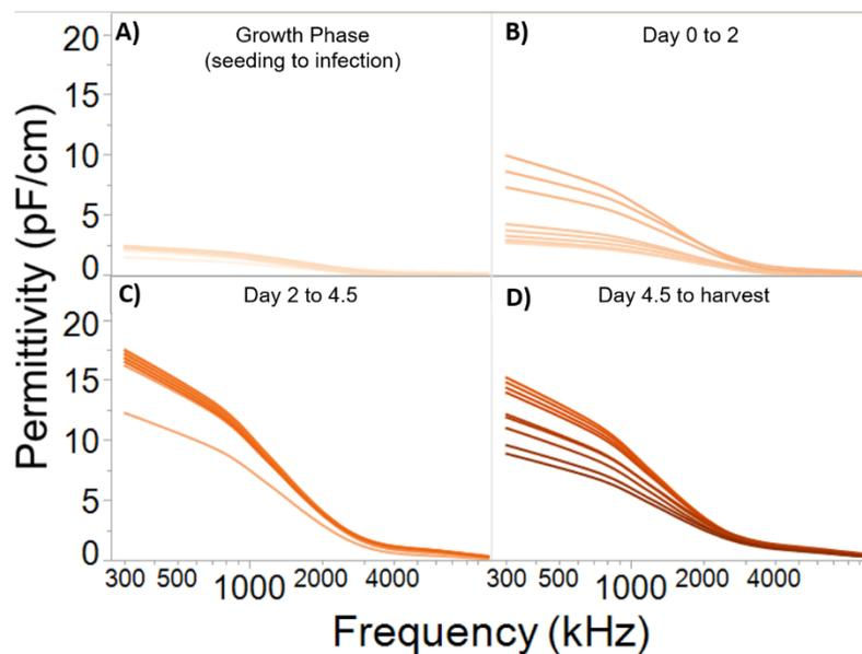
**Figure S2** - Representative beta dispersion curve evolution profiles for different culture phases, here shown for batch number 1. Each curve is colored according to the culture time (the darker the color, the closer the timepoint is to the harvest time). (A) Growth phase (from cell seeding to time of infection). (B) From infection day to day 2 post infection. (C) Day 2 to day 4.5 after infection. (D) Day 4.5 to harvest timepoint.
