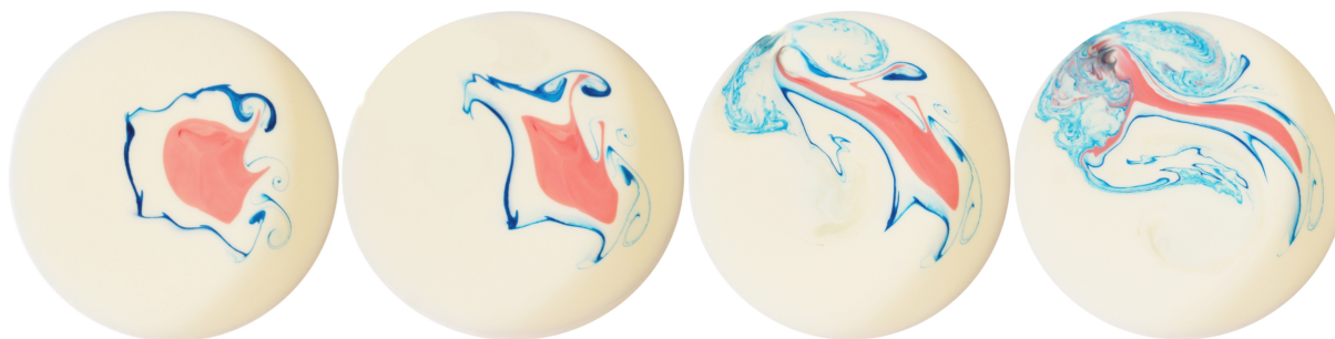
Figure 1. A photograph of the scalar mixing process: three fluids (white, red and blue) arranged on a plate (150 mm diameter) and stirred by a rotating disk (5 mm diameter, 7600 rpm). Pictures taken at about 5 s intervals (courtesy of Zofia Waławczyk (2020)).
