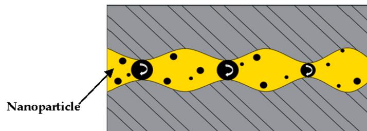
Figure 7. Rolling mechanism by NPs-based lubricant [22].
