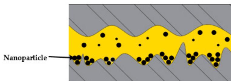
**Figure 10.** Mending effect mechanism by NPs-based lubricant [22].
