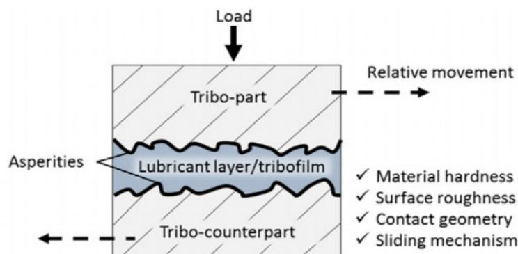
**Figure 2.** Mechanical properties of a tribological system [19].
