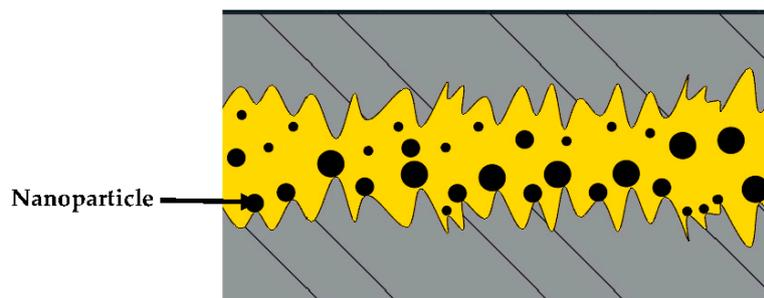
**Figure 12.** Polishing effect mechanism by NPs-based lubricant [22].
