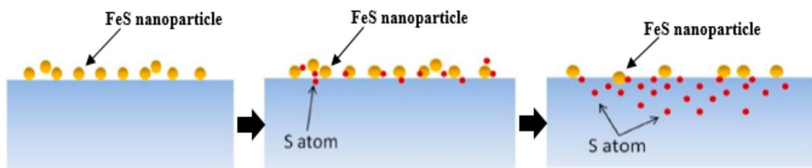
**Figure 6.** Diffusion of S-atom from FeS nanoparticles into the material surface [73].
