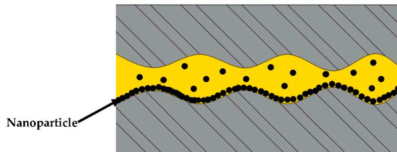
**Figure 8.** Protective film formation mechanism by NPs-based lubricant [22].
