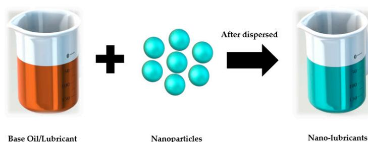
Figure 5. Synthesis of nanolubricants.
