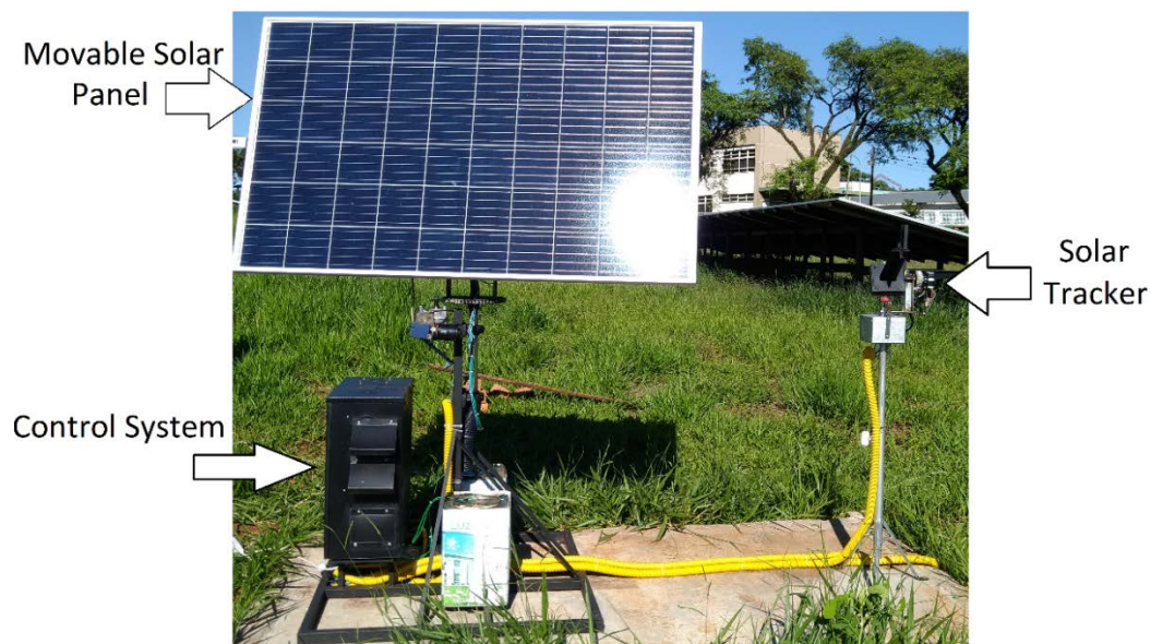
Figure 3. Prototype of two-axis active solar tracker.
