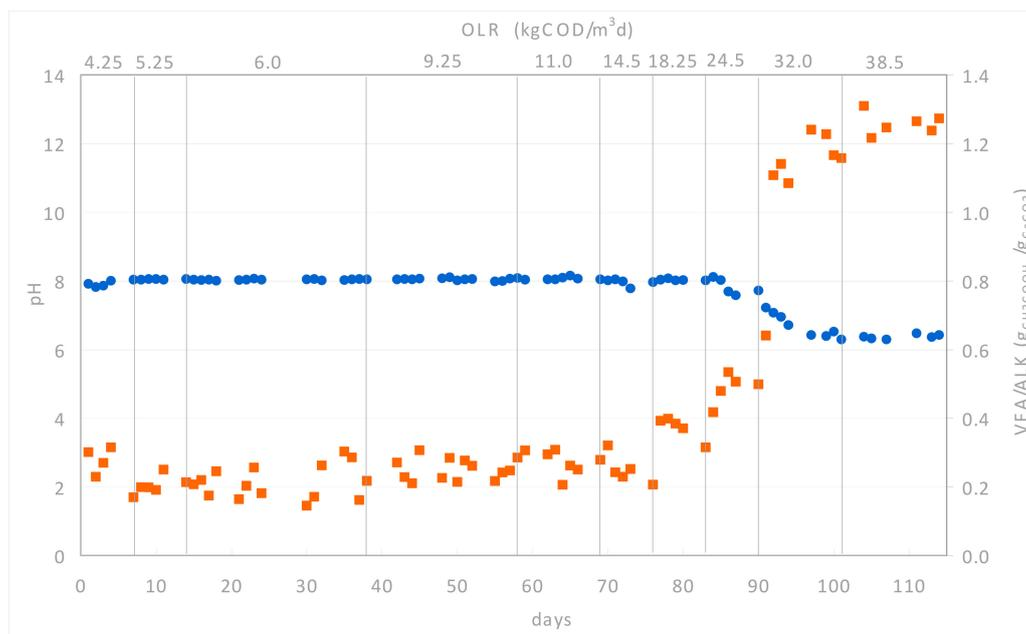
Figure 5. pH and VFA/ALK over the pilot plant operational phase.
