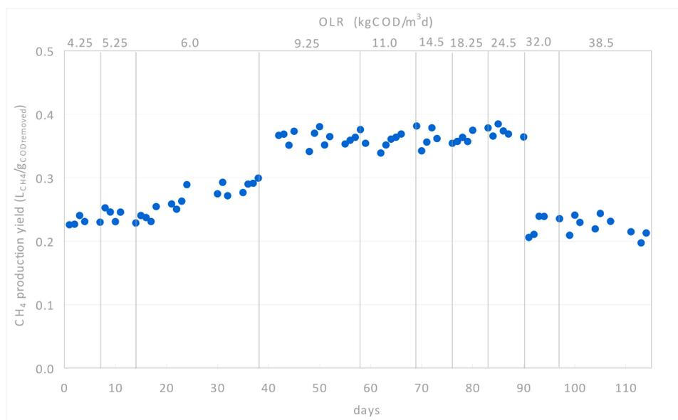
**Figure 4.** Methane production yield over the pilot plant operational phase.
