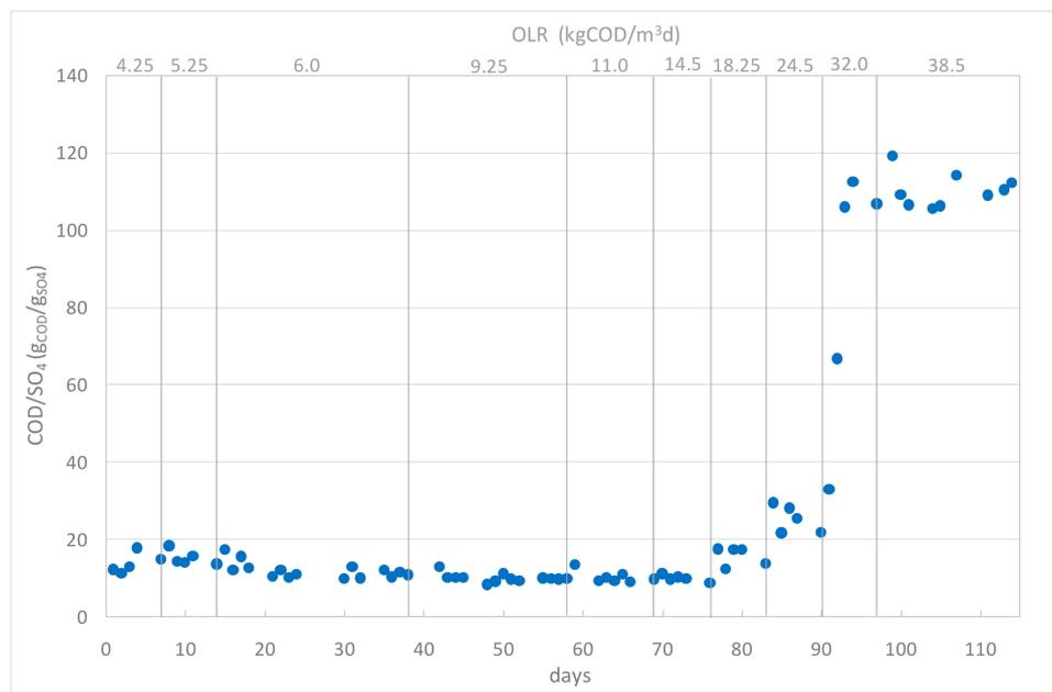
Figure 7. COD/SO<sub>4</sub> ratio over the operational phase of pilot plant.
