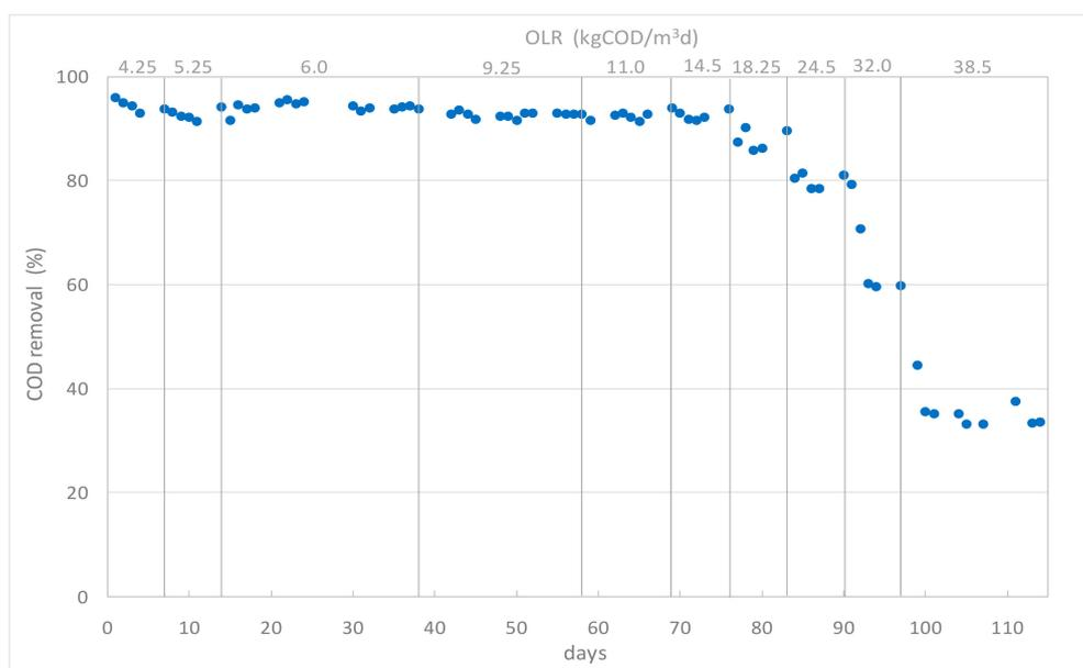
**Figure 2.** Chemical oxygen demand (COD) removal over the pilot plant operational phase.
