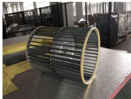
**Figure 22.** Experimental device and impeller model. (a) two-dimensional cross-section of performance measurement device; (b) on-site testing equipment; (c) impeller of model-L in experimental performance measurement.
