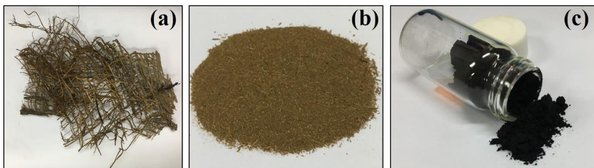
Figure S1. (a) shows the raw I-DPF, (b) shows the I-DPF after grinded and sieved (size less than 1 mm) and (c) I-DPF after activation (bio-PAC).
