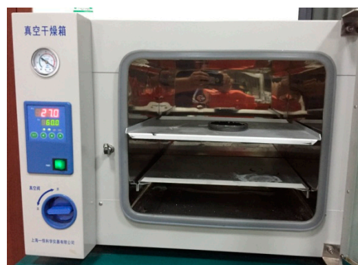
Figure 1. Vacuum drying chamber with a preset temperature.
