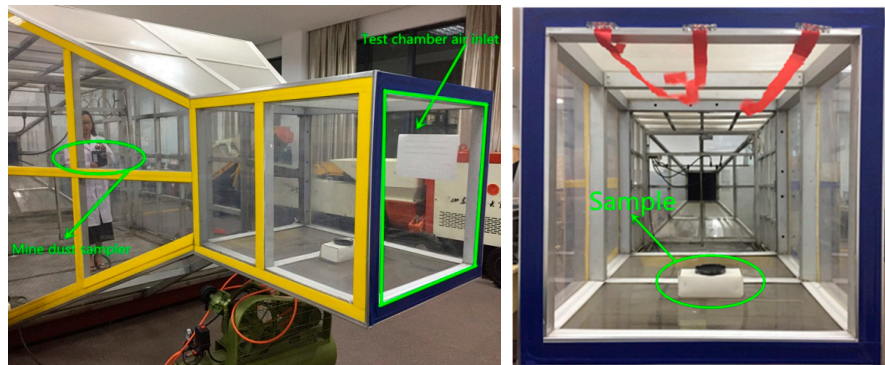
Figure 5. Air tunnel simulation apparatus.
