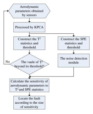
Figure 1. Process of fault diagnosis and location.
