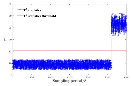
**Figure 6.** Value of the T<sup>2</sup> statistic under the condition of an LPT fault.
