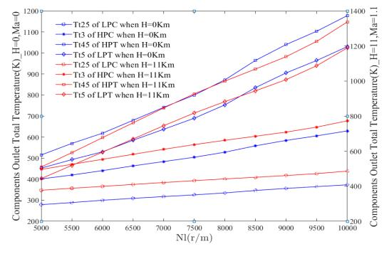
**Figure 2.** Total temperatures of components.
