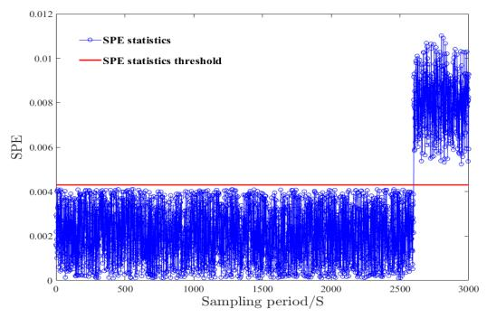
Figure 5. Value of SPE statistic under the condition of LPC fault.
