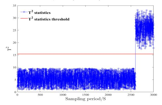
Figure 4. Value of the T<sup>2</sup> statistic under the condition of an LPC (low pressure compressor) fault.
