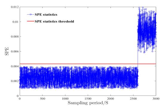
Figure 7. Value of the SPE (Squared Prediction Error) statistic under the condition of an LPT fault.
