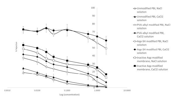
Figure 10. Rejection trends for Sodium chloride and calcium chloride filtration.
