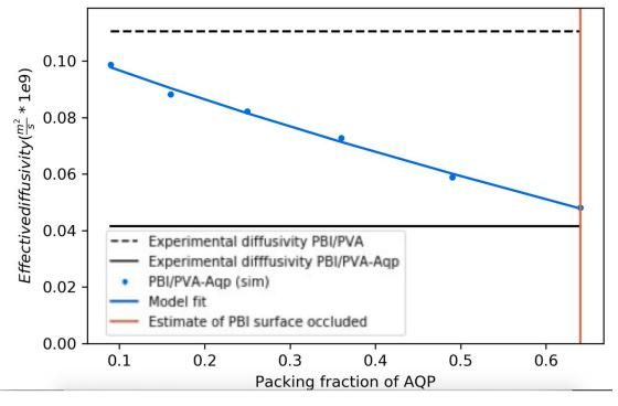
**Figure 11.** Predictions and experimentally measured effective diffusion coefficients, based on the geometry in Figure 4. Black lines correspond to experimental data found in Supplemental Table S1. Blue lines represent aggregate (solid) and monomeric (dots) Aqp models, respectively.
