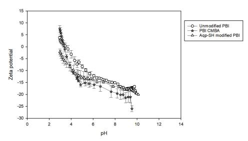
**Figure 7.** Zeta potential values of unmodified PBI, PBI-CMBA, and Aqp-SH modified PBI membranes over a pH range of 2–10.
