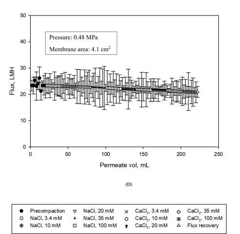
**Figure 9.** (**A**): Flux analysis of unmodified PBI membrane; (**B**): Flux analysis of PVA-alkyl modified PBI membrane; (**C**): Flux analysis of inactive Aqp-SH modified PBI membrane; and (**D**): Flux analysis of Aqp-SH modified PBI. All flux analyses were carried out at constant pressure of 0.48 MPa (4.83 bar). Five concentrations each of NaCl and CaCl<sub>2</sub> solutions were used as feed solutions and reverse flow filtration was used after every solution filtration.
