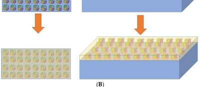
**Figure 1.** (**A**) Cys modified aquaporin molecule (Aqp-SH). (**B**) Chemical attachment of Aqp-SH on –COOH modified Polybenzimidazole (PBI-COOH) membrane and in-situ addition of a layer of Polyvinyl alcohol carrying long alkyl chains (PVA-alkyl).
