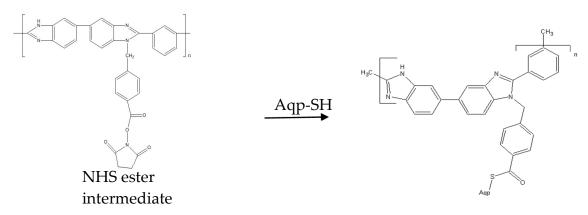
**Figure 3.** Chemical attachment of Aqp-SH to –COOH modified PBI membranes using carbodiimide chemistry.
