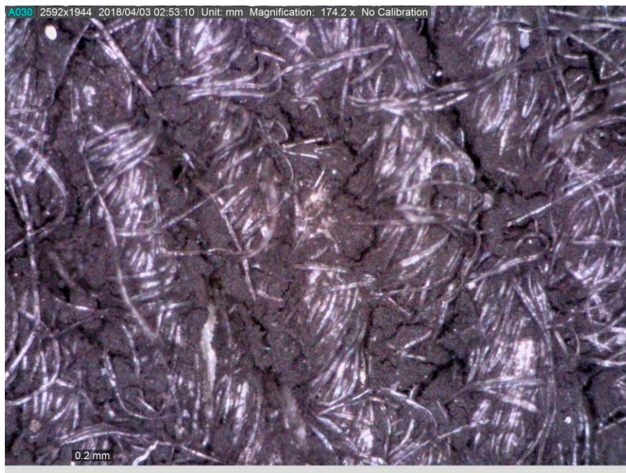
Figure 8. Surface views of a control with no fungal exposure (a), as well as control (b) and NW-40% (c) specimens after being exposed to A. niger .
