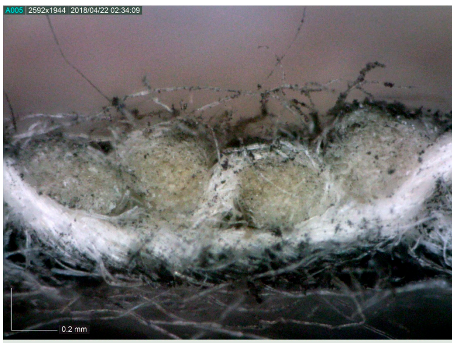
Figure 8. Surface views of a control with no fungal exposure (a), as well as control (b) and NW-40% (c) specimens after being exposed to A. niger .
