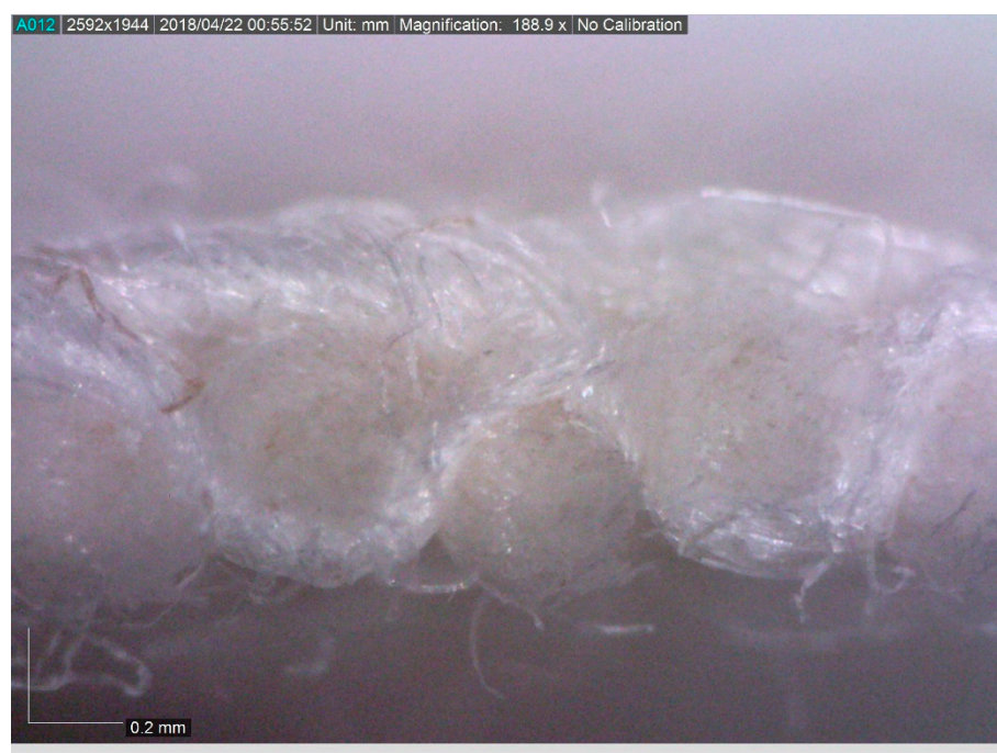
Figure 7. Cross-sectional of control textile specimen showing large cavities in between fibers for transfer of fluid.
