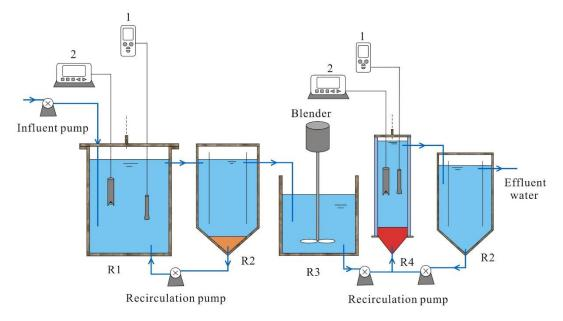
**Figure 1.** Schematic of experimental setup. Influent pump, influent water pump; recirculation pump, reflux water pump; R1, partial nitrification reactor; R2, sedimentation/adjustment tank; R3, transfer tank; R4, anammox reactor; 1, pH online monitoring; 2, DO online monitoring.
