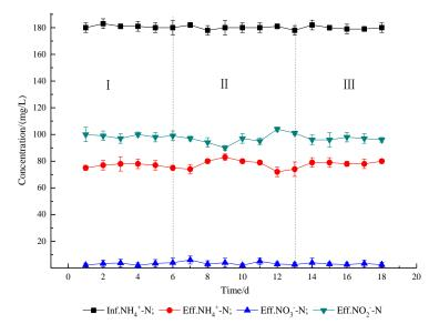
**Figure 2.** Nitrogen relationship between influent and effluent during the partial nitrification stage; Stages I, II, and III indicate that HRT is 14, 10, and 6 h, respectively.
