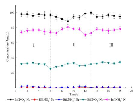
**Figure 5.** Nitrogen relationship between influent and effluent in anammox; Stages I, II, and III indicate that HRT is 33.4, 24, and 14.5 h, respectively.
