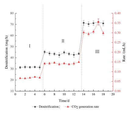
**Figure 7.** Relationship between CO<sub>2</sub> consumption and amount of denitrification in anammox; Stages I, II, and III indicate that HRT is 33.4, 24, and 14.5 h, respectively.
