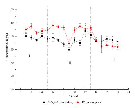
**Figure 3.** Relationship between inorganic carbon (IC) consumption and NO<sub>2</sub><sup>-</sup>-N production in partial nitrification; Stages I, II, and III indicate that HRT is 14, 10, and 6 h, respectively.
