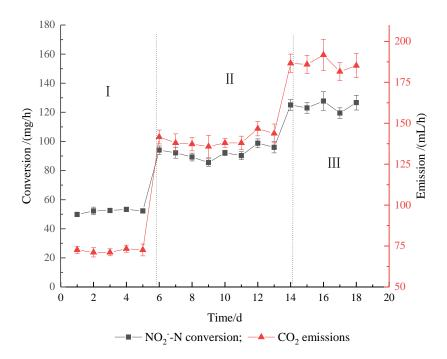
**Figure 4.** Relationship between CO<sub>2</sub> emissions and NO<sub>2</sub><sup>-</sup>-N conversion during the partial nitrification stage; Stages I, II, and III indicate that HRT is 14, 10, and 6 h, respectively.
