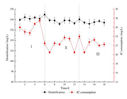
**Figure 6.** Relationship between inorganic carbon (IC) consumption and the amount of denitrification in anammox in hydraulic retention time (HRT) experiments; Stages I, II, and III indicate that HRT is 33.4, 24, and 14.5 h, respectively.
