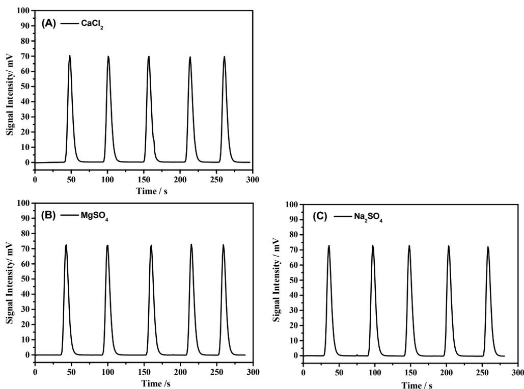
**Figure 7.** Adsorption performance of desiccants on CO<sub>2</sub> tested with pulse adsorption, (A) CaCl<sub>2</sub>, (B) MgSO<sub>4</sub>, (C) Na<sub>2</sub>SO<sub>4</sub>.
