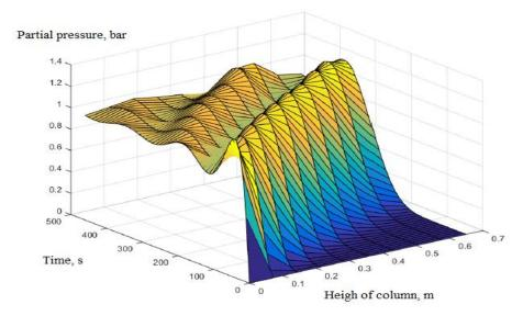
$\textbf{Figure 4.} \ \ \text{The result of partial pressure (O}_2) \ \ \text{following over time and height of column at 5 bar.}$
