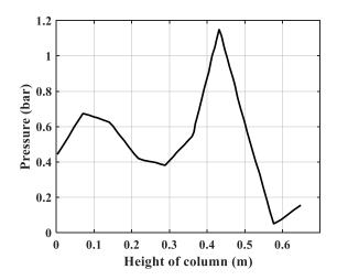
**Figure 8.** The result of partial pressure (O<sub>2</sub>) following height of column at 5.5 bar.
