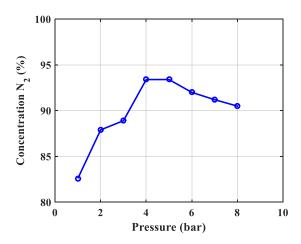
Figure 19. The dependence of  $\ensuremath{N_2}$  concentration on adsorption pressure.
