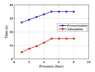
Figure 17. Adsorption time depends on adsorption pressure.
