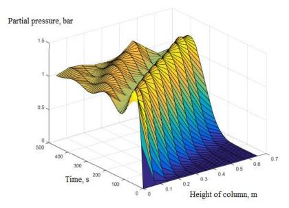
**Figure 7.** The result of partial pressure (O<sub>2</sub>) following over time and height of column at 5.5 bar.
