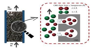
Figure 1. Selective adsorption mechanism of CMS material.
