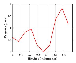
**Figure 11.** The result of partial pressure (O<sub>2</sub>) following height of column at 8 bar.
