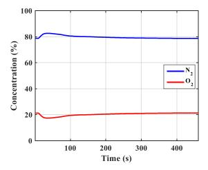
**Figure 15.** Concentration of gas N<sub>2</sub> at the output of a single fixed bed (see Figure 2).
