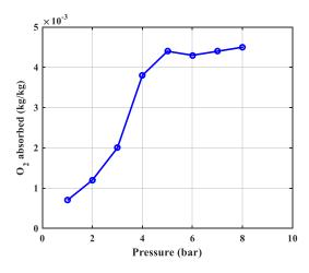
Figure 20. The amount of O2 gas absorbed depends on the pressure.
