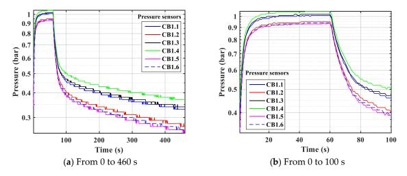
Figure 13. Pressure over time and heigh of a single fixed bed (see Figure 2).
