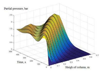
Figure 10. The result of partial pressure (O<sub>2</sub>) following over time and height of column at 8 bar.
