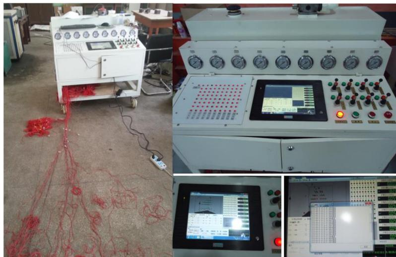
**Figure 3.** The visualization platform of the grouting diffusion.
