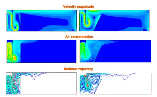
Recent systematic theoretical analyses clearly depicted the various hydrodynamic and physicochemical parameters that dictate flotation performance The application of CFD codes to simulate large-scale flotation processes offers distinct advantages in investigating the relative significance of various design
