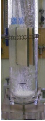
Typical selected results, while membrane backflushing testing, are presented in Figure 9; for *Saccharomyces* yeast removing zinc ion [67]. As the unit also needs periodic backflushing for efficient operation. Flotation removed effectively a major part of the biomass particles, responsible for membrane fouling.
