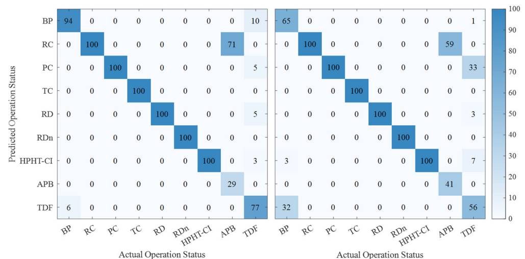
Figure 6. Confusion matrix illustrating the classification performance of the SVM model for nine drilling operation statuses under (left) s = 0 ; (right) s = 1 . Results are based on [0, 1] normalization and t = 2 . Abbreviations correspond to Table 1.
