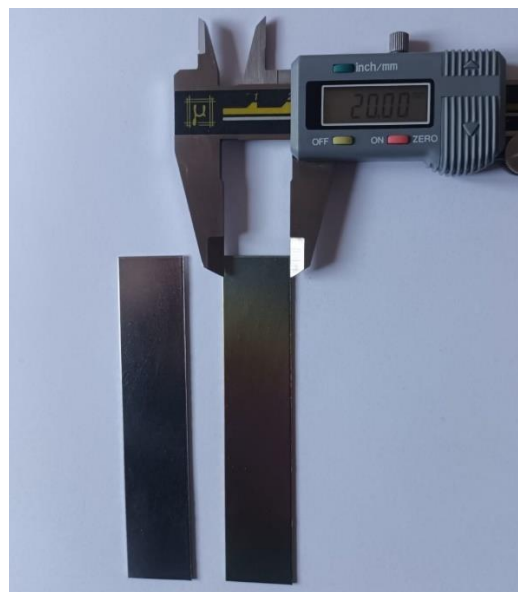
Figure 2. Ni-Ti SMA before (left image) and after (right image) shape setting heat treatment.
