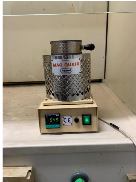
Figure 1. Electric furnace with digital temperature control used for the shape setting of Ni-Ti SMA.
