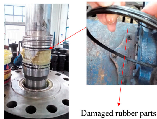
Figure 3. Failure of the rubber ring after the test.
