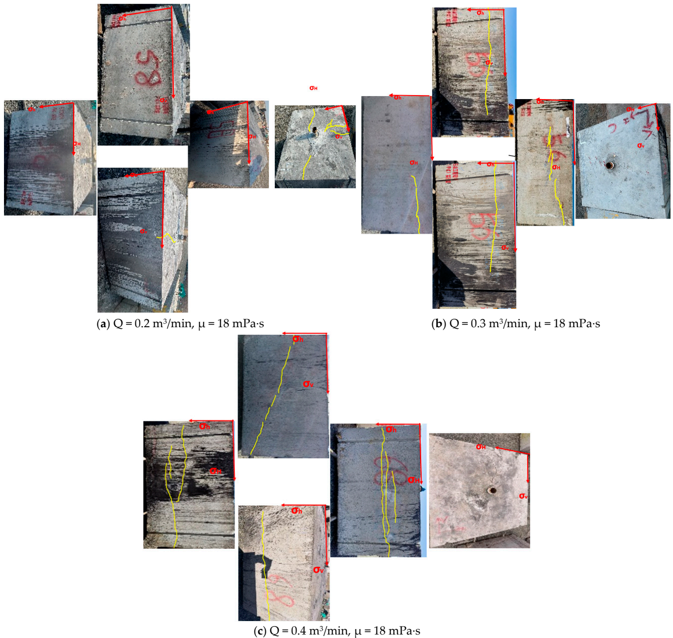
Figure 3. Crack Distribution at Different Displacement Levels. (Non-English term: Petroleum Engineering Field (Pilot) Laboratory).
