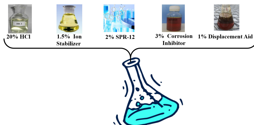
Figure 2. The new acidizing solution formula.
