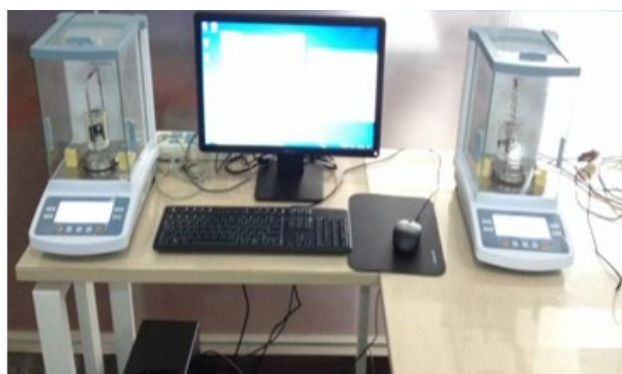
Figure 4. Spontaneous imbibition measurement system diagram.
