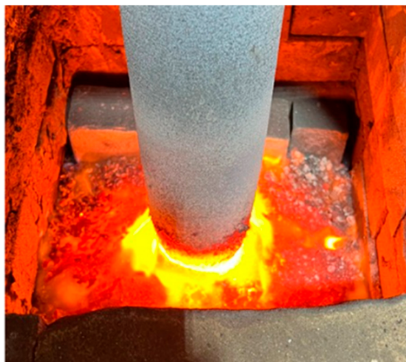
Figure 10. SiC synthesis process: view of the furnace throat with crushed charge.
