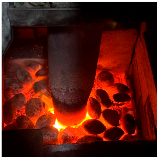
Figure 7. SiC synthesis process: view of the furnace throat.
