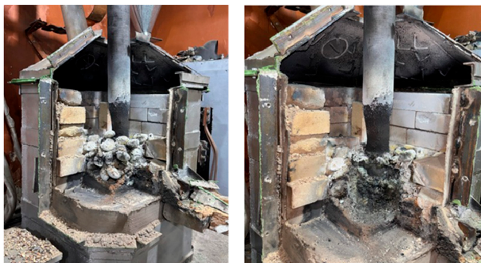
Figure 8. View of the dismantled furnace after synthesis.
