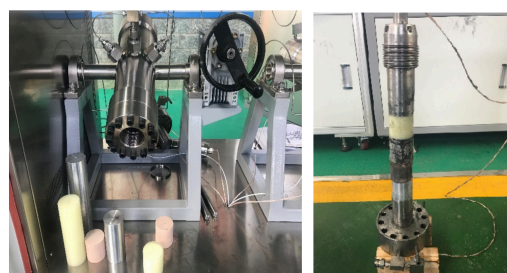
Figure 9. Steel block simulated cylindrical rock sample test.
