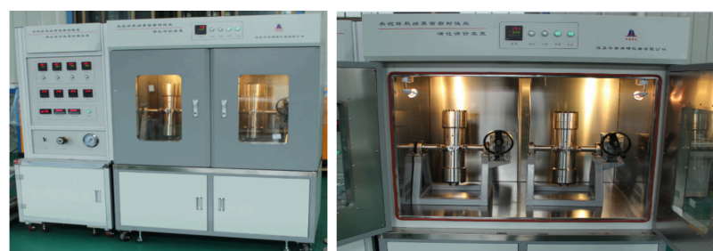
Figure 5. Evolution evaluation device for sealing ability of the cement–formation interface of cement ring bonding.
