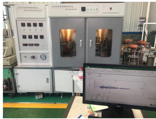
Figure 6. Sealing acoustic test platform at the second cementing interface.
