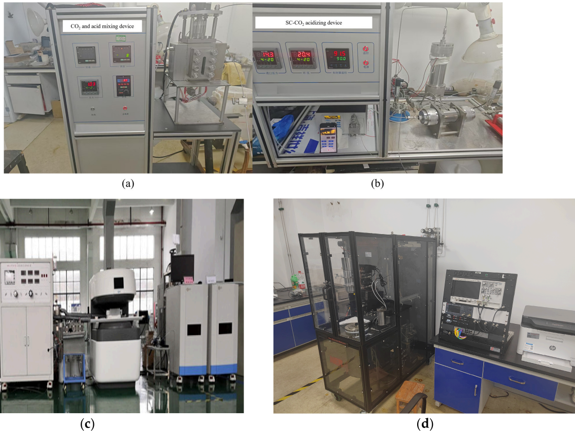
Figure 6. Experimental device. (a) CO 2 and acid mixing device; (b) SC-CO 2 acidizing device; (c) core NMR testing device; (d) porosity–permeability testing device.
