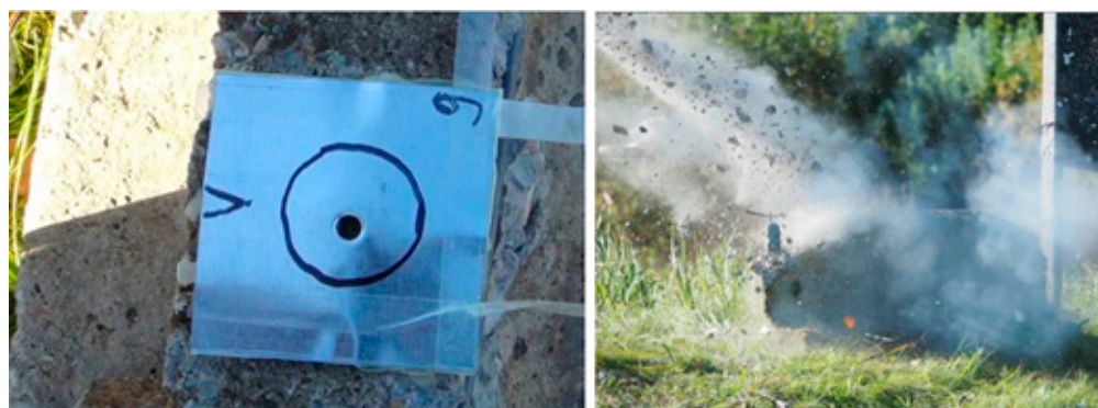
Figure 5. Preliminary investigation of the reaction of 3-picrylamino-1H-1,2,4-triazole (on the left) to 7.62 mm bullet impact. Control sample of TAGN detonated after bullet impact in current conditions (on the right).
