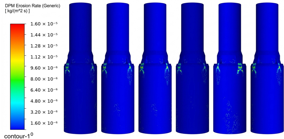
Figure 8. Erosion-rate distribution under different inlet flow capacities.
