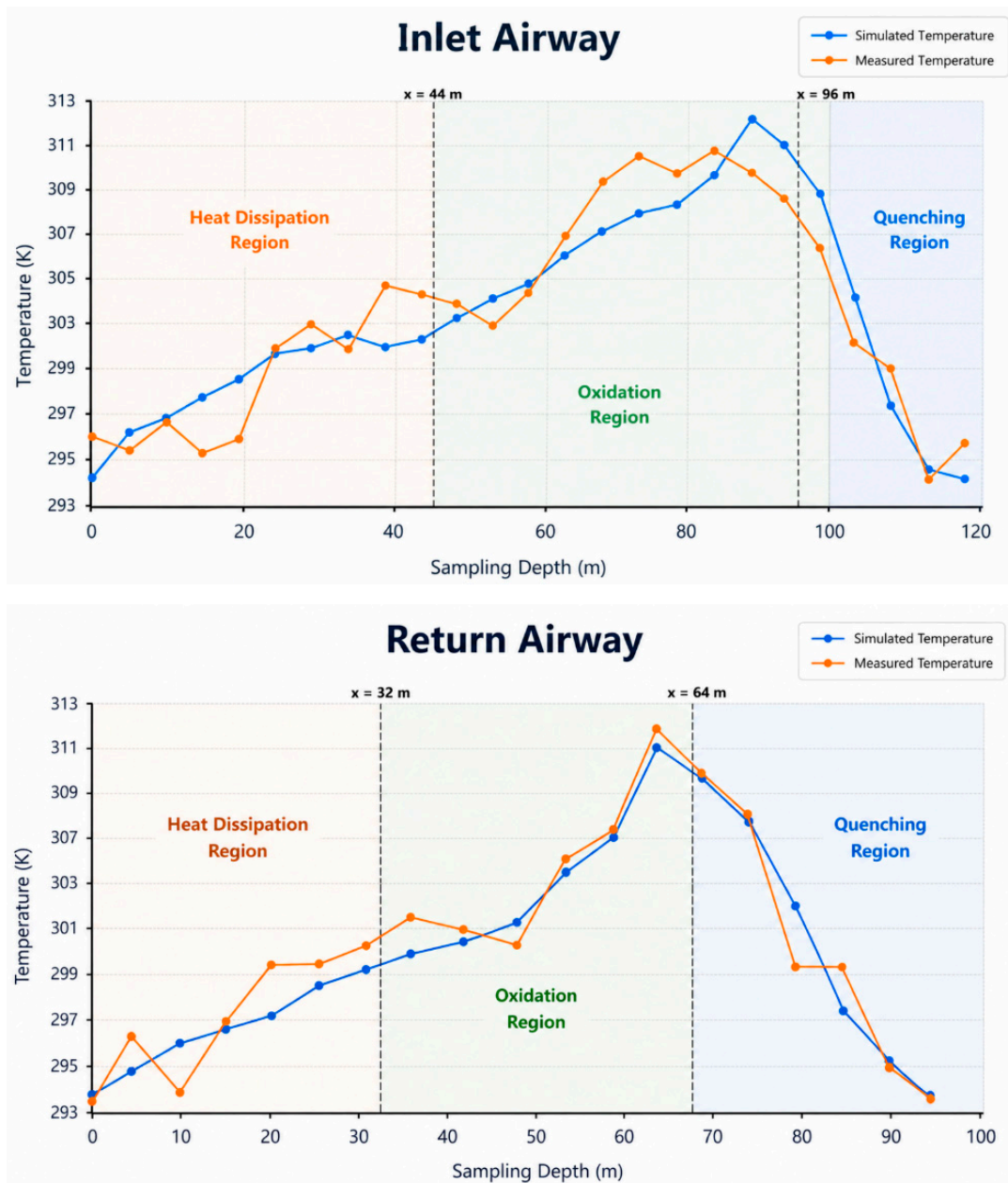
Figure 17. Comparison of simulated and measured temperatures on both sides of the goaf.
