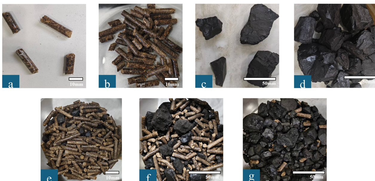
Figure 1. Typical visual characteristics of coal, biomass, and blended samples under different blending states: (a) biomass particles with low stacking density; (b) biomass particles with high stacking density; (c) coal particles with low stacking density; (d) coal particles with high stacking density; (e) low-coal-fraction blended sample; (f) medium-coal-fraction blended sample; (g) high-coal-fraction blended sample. Scale bars are shown in each panel.
