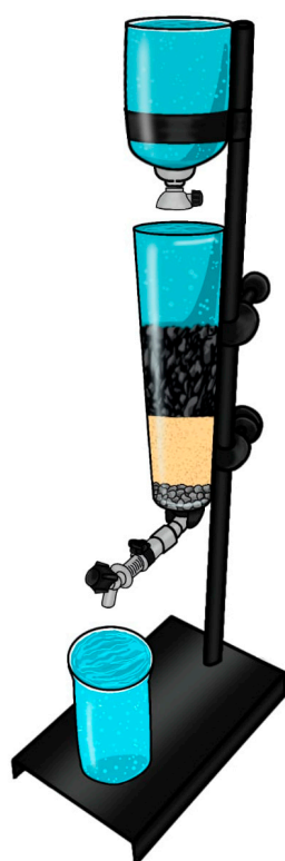
Figure 2. Design of the rapid downward-flow dual-media filter.
