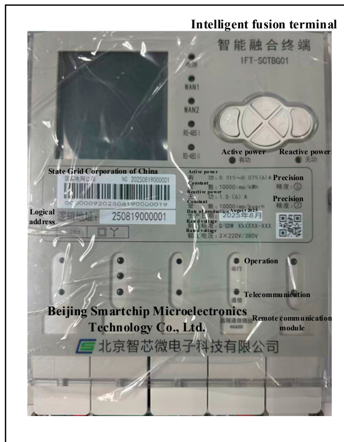
Figure 6. Schematic diagram of the smart terminal.
