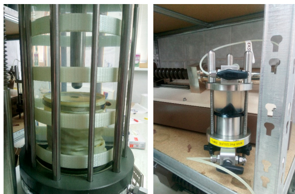
Figure 2. Triaxial cell with installed sample ( left ), toxic cell ( right ).
