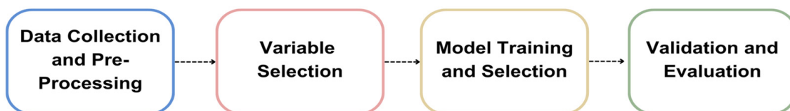
Figure 5. Soft-sensing framework for real-time bioprocess monitoring.
