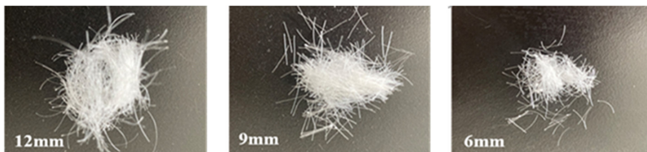
Figure 2. Schematic diagram of three polyester fibers with different lengths.
