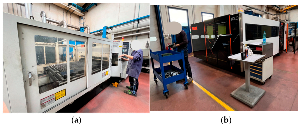
Figure 2. Monitored laser cutting devices: (a) CO 2 laser device; (b) Fiber laser device.
