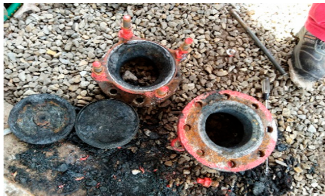
Figure 1. Structural illustration of the field-installed flame arrester.
