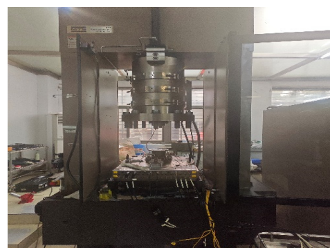
Figure 5. MTS815 pressure testing system.
