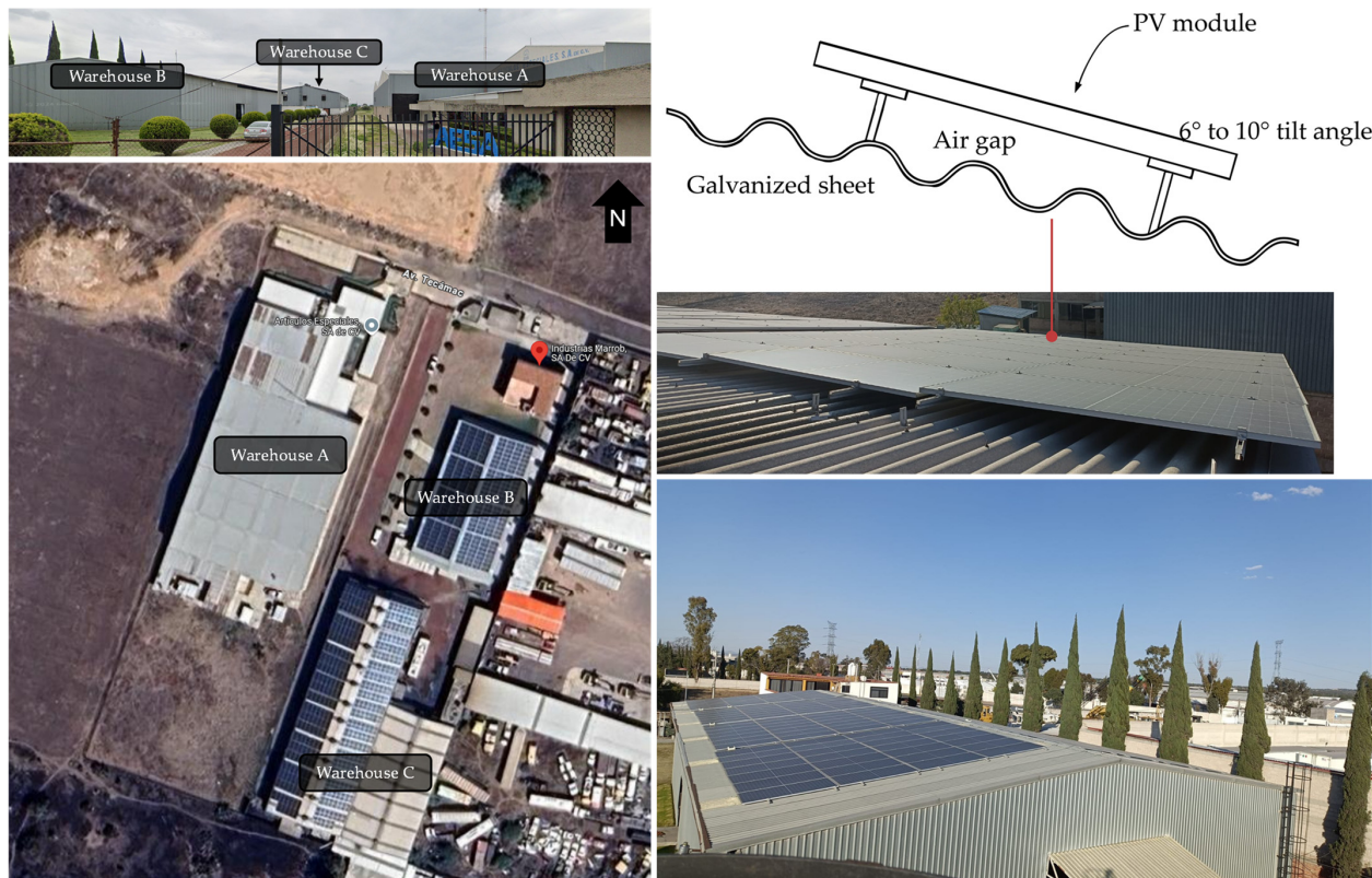
Figure 1. Site and photovoltaic configuration. Left: aerial view of the study facility in Tecámac, Estado de México, identifying Warehouses A (no PV), B (full-roof PV), and C (full-roof PV). Right, top to bottom: schematic roof section showing PV module mounted parallel to the corrugated galvanized sheet with a 0.10 m air gap at the roof pitch (6–10°); close-up photograph of the module standoff; and oblique photograph of the fully covered roof of Warehouse B.
