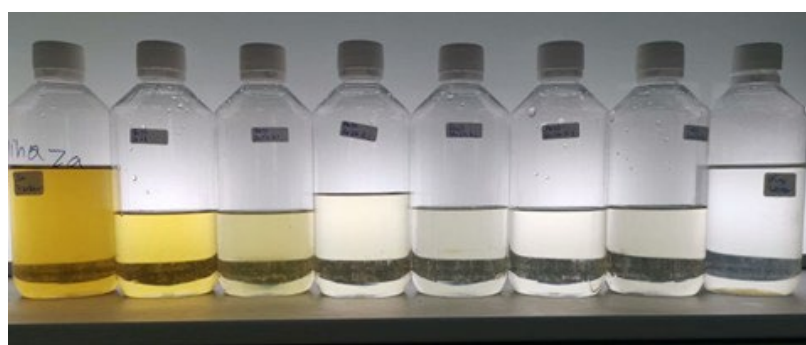
Figure 3. Voltage effect for 2 h treatments. From left to right: pretreated vinasses, 1 V, 2 V, 3 V, 4 V, 5 V, 6 V, and pure water.
