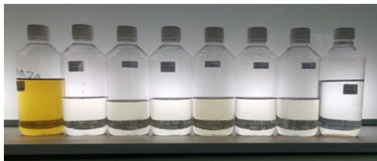
Figure 12. Time effect for 5 V treatments. From left to right: pretreated vinasses, 1 h, 2 h, 3 h, 4 h, 5 h, 6 h, and pure water.
