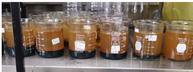
Figure 21. Sludge volume yield after two hours of treatment with variable voltage. From left to right: 6 V, 5 V, 4 V, 3 V, 2 V, and 1 V.
