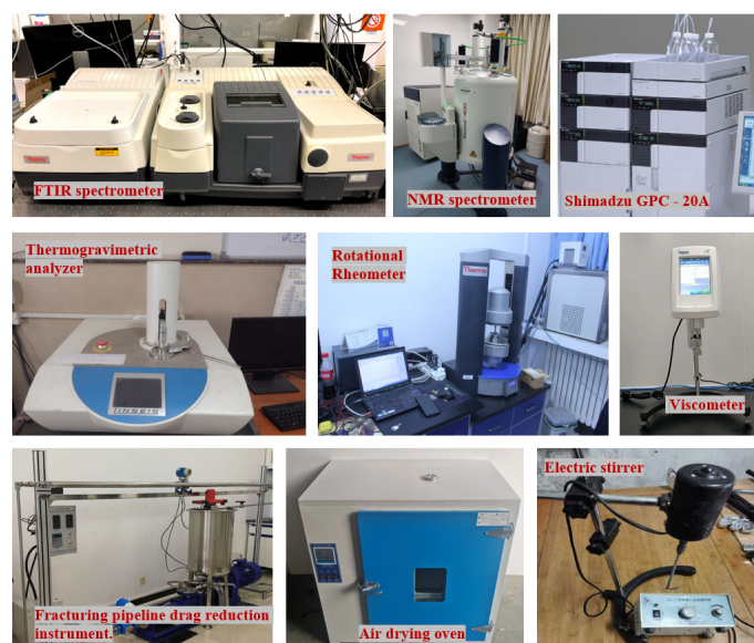
Figure 1. Experimental apparatus physical diagram.
