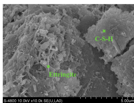
Figure 11. The C-S-H gel and Ettringite minerals formed in the interception materials layer.
