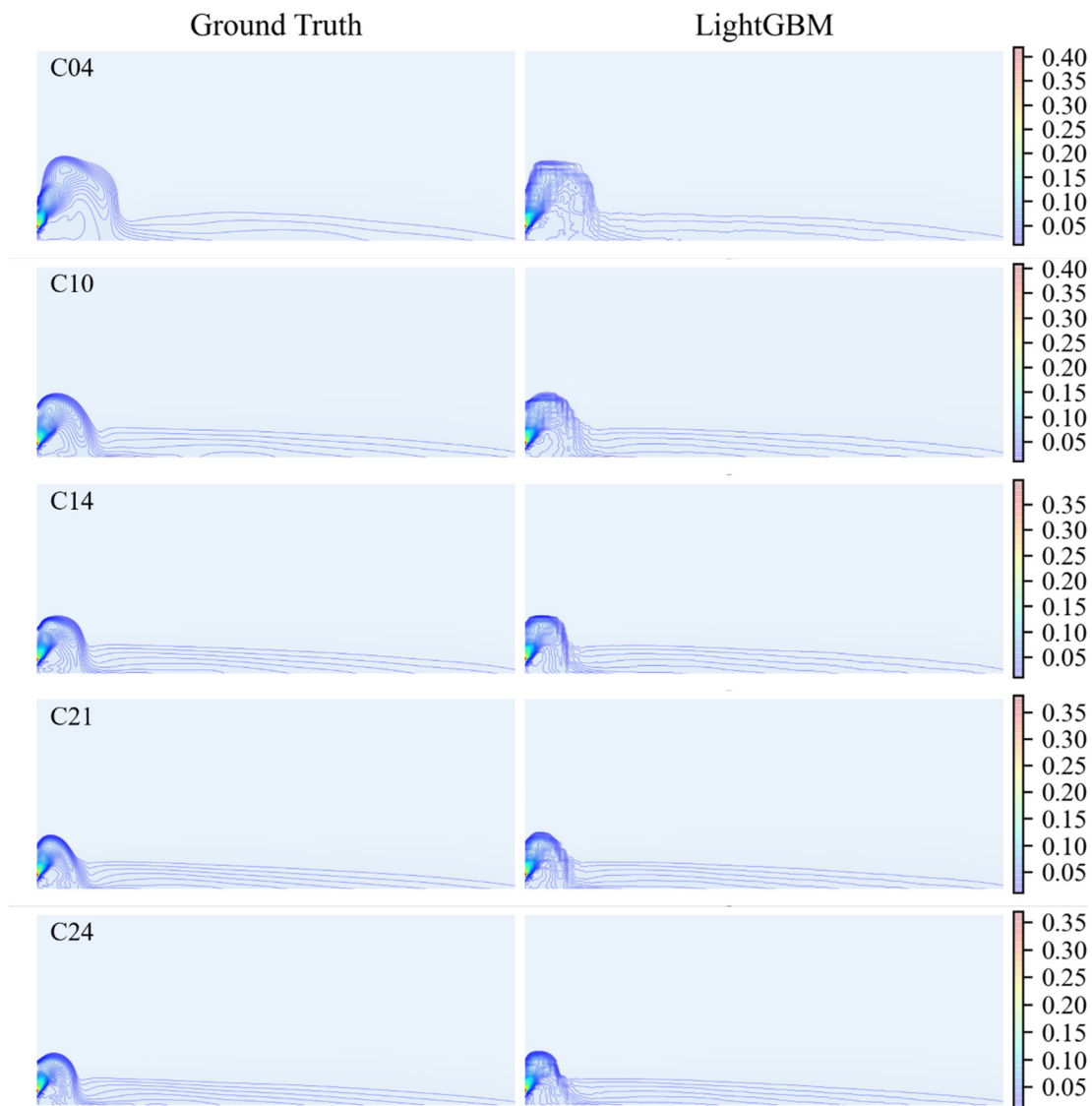
Figure 6. Comparison of the LightGBM model and the ground truth concentration field distribution in the unseen data.
